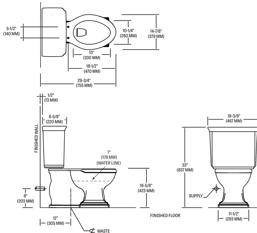
Fixture performance and specifications meet or exceed ASME A112.19.2-2013/CSA B45.1-13 standards, and other state and local codes.
